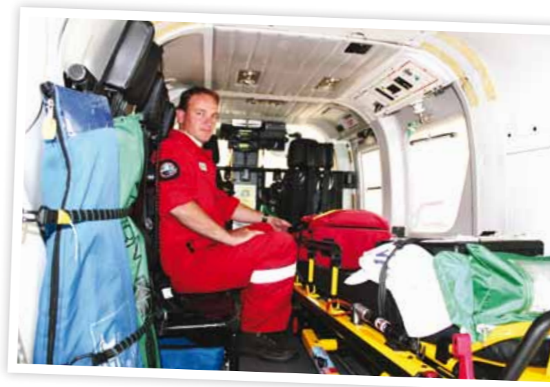
Lowe Corporation Helicopter Rescue Service pilot Dean Herrick inside the BK117 helicopter, showing the fold-up stretcher at right and paramedic seats that can be used in an emergency as a stretcher bench for a second patient.
